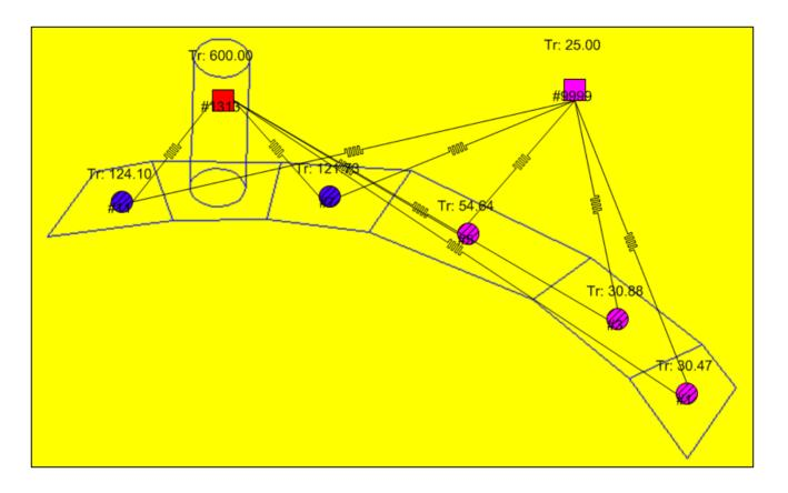
The radiation conductors between surfaces are computed by Nevada and the thermal results obtained by SINDA/G.
