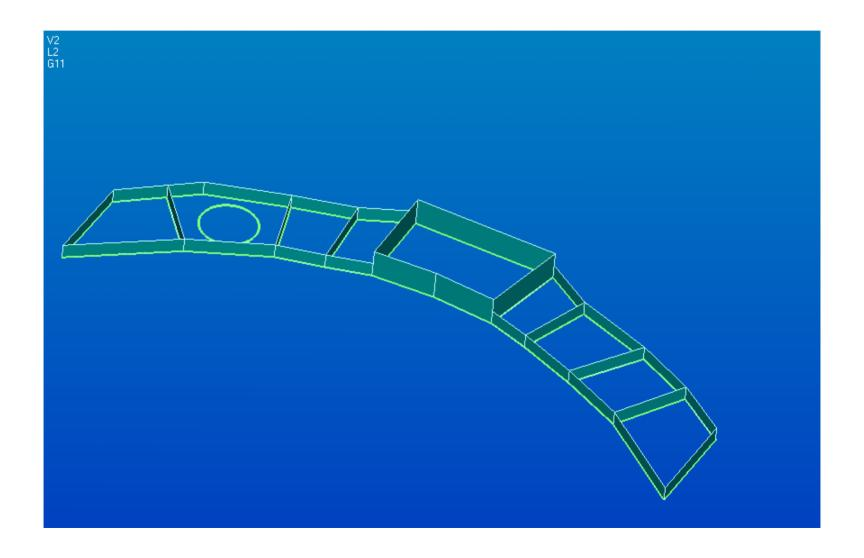
The surfaces are then individually meshed and elements interconnected by using node merge command.
