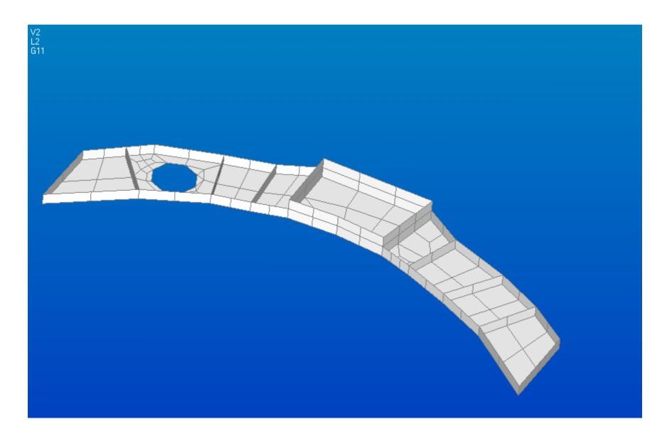
The pipe was meshed boundary conditions applied and the model analyzed.
